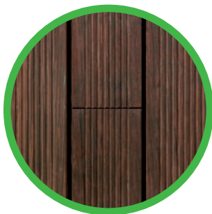
New, non-weathered decking
