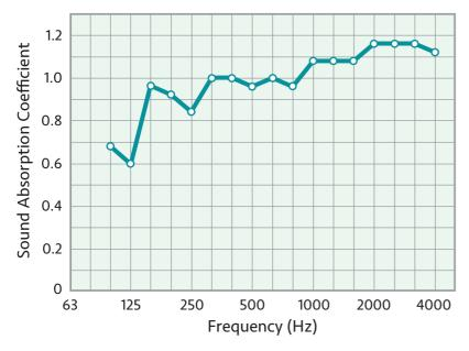
Noise Reduction Coefficient: NRC = 1.00 In accordance with EN ISO 11654:1997, Weighted Absorption Coefficient,  $\alpha_w = 1.00$ Sound absorption class is A.
