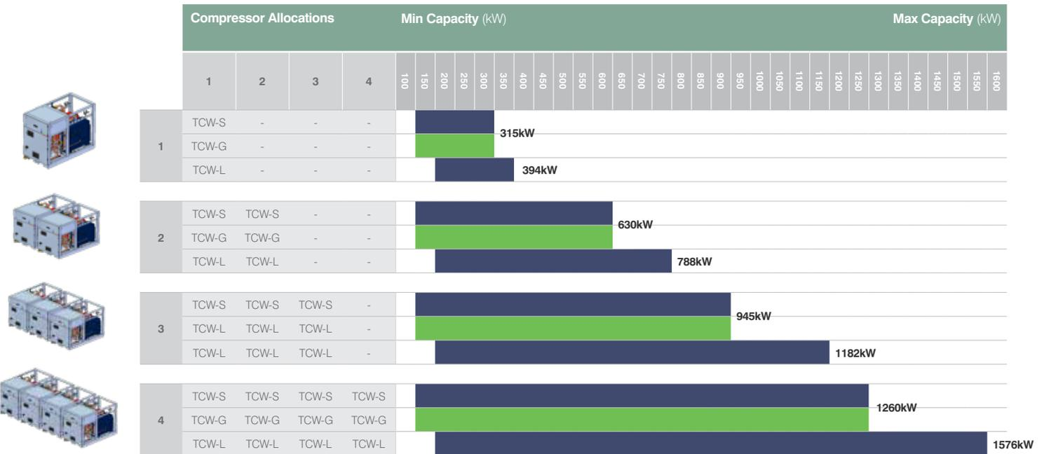
\* Based on nominal design conditions 12/7°C Evaporator water , 30/35°C Condenser water
