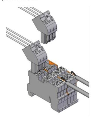
The plugged termination ensures that the connections are made simultaneously. Failure to attach the cables this way may cause damage to the controller.
