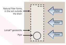
Geotextile wrapped filter drain
