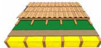
Warm RoofTile with OSB Detail
