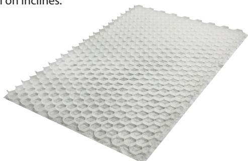
Both the large sheet (2400x1200mm) and the small sheet (1200x800mm) come with an 80gsm non-woven weed membrane heat welded to the underside of the grid. This not only prevents weed growth from beneath the surface, but also prevents the gravel from migrating under the cell wall and into the sub base over time.
