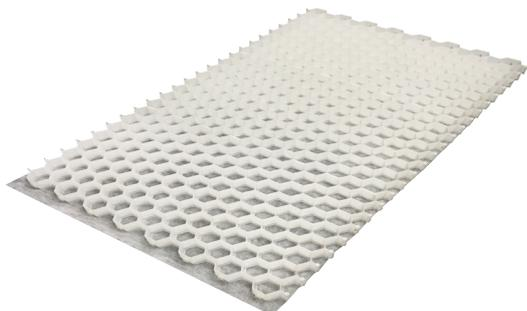
Both the large sheet (2400x1150mm) and the small sheet (1150x800mm) come with a 50gsm non-woven weed membrane heat welded to the underside of the grid. This not only prevents weed growth from beneath the surface, but also prevents the gravel from migrating under the cell wall and into the sub base over time.
