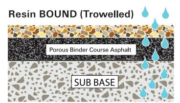
Top surface: **15 -18mm** thick 'bound' mixture of stones and resin
