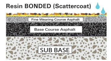
Top surface: **3mm** layer of single stones 'bonded' to resin
