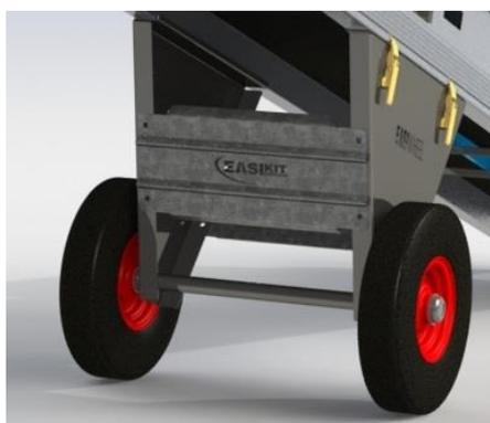
3. Secure in place tightening the four over-centre catches.
