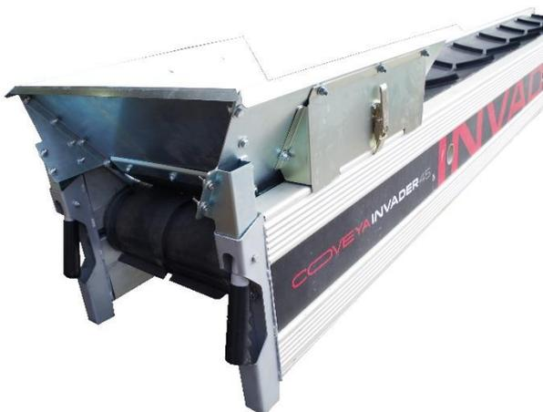
1. Fit the hopper to the loading end of the conveyor. Align the locating posts and secure the hopper to the conveyor by means of the two over-centre catches.
