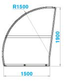
DIMENSIONS: Width: 1500mm Length: 3600mm Height: 1900mm
