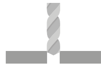
6.5mm diameter fig.14 – Sliding point
