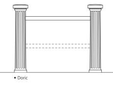
We generally recommend that rails are Ø48mm tube for spans of approximately 1000mm. Only bollards of appropriate diameter at the rail insertion pont are suitable for use as cycle stands.
