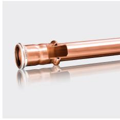
Geberit Mapress is a metal pressing system that provides an efficient, safe, and reliable solution for a range of different job requirements. To ensure a safe and long lasting connection the fitting and pipe are pressed once the pipe has been inserted to the required insertion depth.
