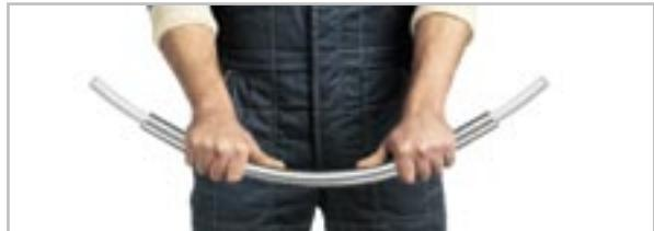
**Important:** Do not use a bending spring on the inside! iFIT tools must be used!
