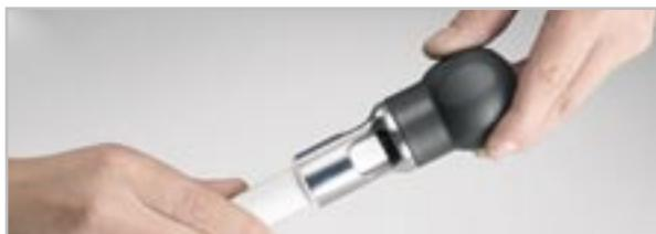
2. Calibrate and deburr pipe with hand tool.
