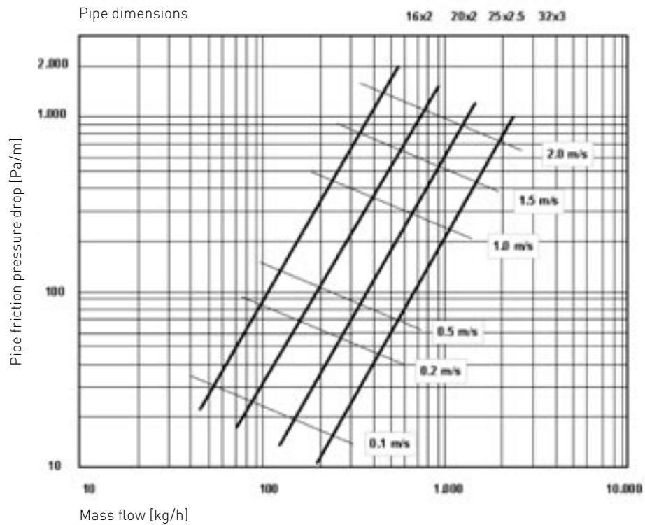
Pipe friction pressure drops in relation to mass flow at an average heating temperature of 60°C.
