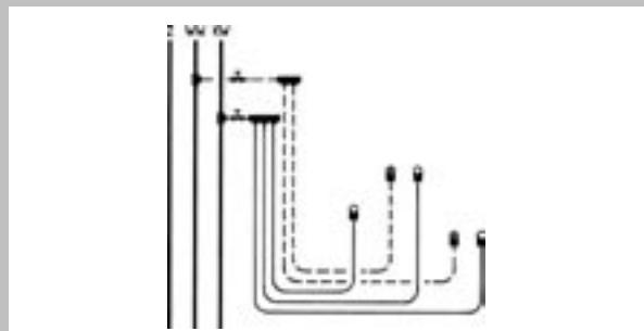
Individual feed pipes supply only one water
