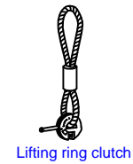
Detail 'A' 'Cast in' Universal anchor point
