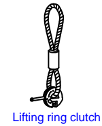
Detail 'A' 'Cast in' Universal anchor point
