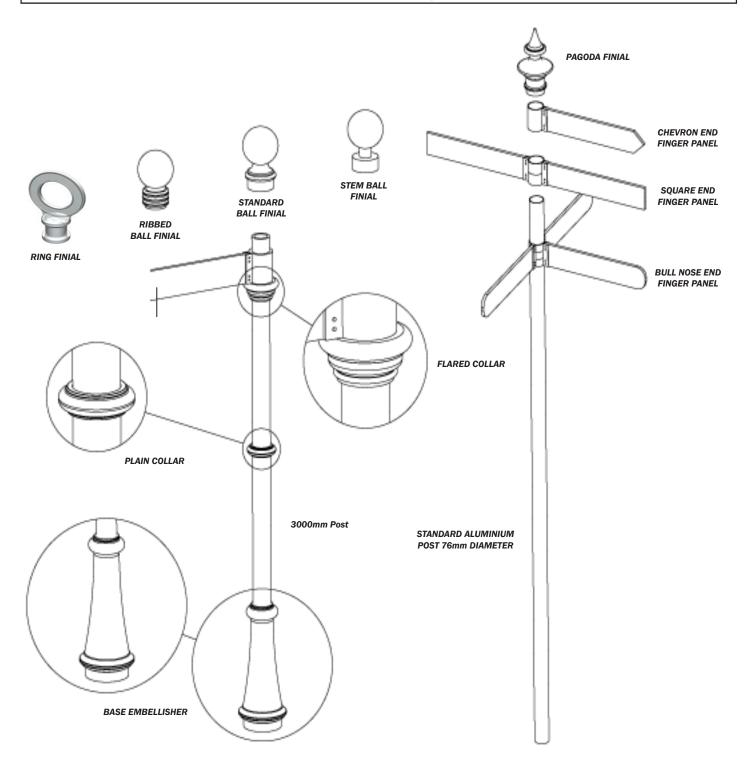
Finger panels can be arranged in any direction by simply rotating through 360 before locking in place.
