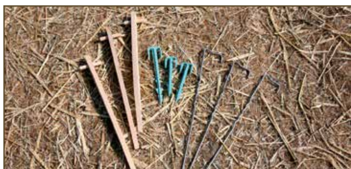
18.1 Variety of fixing pins to meet various soil conditions
