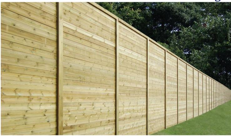
A lighter 20mm thick board than our other Jakoustic® barriers, maintaining the same 125mm cover face. Planed Tongue and Grooved boards with small chamfers which form a "V" join between boards. Suitable for installation where the required noise reduction is lower than that which would provided by the standard Jakoustic® noise barrier - or where a superficial mass of 10, 11 or 12kg/m² is specified.
