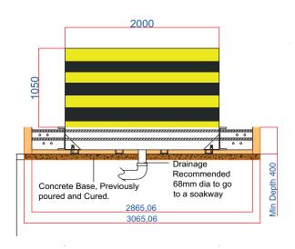
The Crash Rated Shallow Mount Road Blocker has been designed to prevent the threat of potential terrorist attacks where high security is required.
