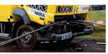
In the UK it is PAS 68, a standard introduced in 2005. In mainland Europe, CWA 16221 has been applied since 2010. In the USA, the ASTM F2656 standard has progressively taken over from the Department of State's 'K' ratings.
