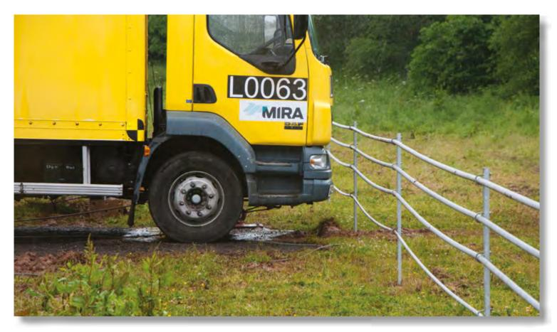
The Linebacker<sup>®</sup> PAS 68 Shallow Foundation is a cable type crash fence that has been successfully impact tested in accordance with BSI PAS 68:2010 to stop a 7.5 tonne vehicle travelling at 50 mph (80km/h). Its shallow foundations allow the fence system to be deployed in sites with utility congested substructures and underground services.
