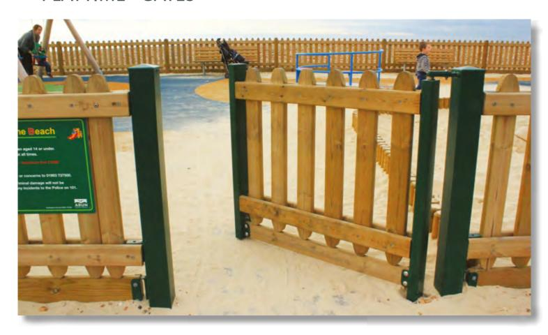
Designed to complement our Timber Playtime® and Metal Playtime® fencing, Playtime® gates conform to all current play area safety guidelines. Gates come complete with hinges that allow the gate to swing through an angle of 180° and 90° if a self closer is added. The hinges are fully adjustable with tamper-proof screws and bolts.
