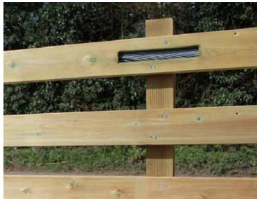
Linebacker PNR features the PAS 68 certified and Secured by Design preferred Linebacker crash fence system, concealed within a traditional timber post and rail fence design. Jacksons Linebacker has been successfully impact tested in ac-cordance with BSi PAS 68:2010, PAS 68 rating of PAS 68:2010 V/7500(N3)/80/90:7.3/21.4)
