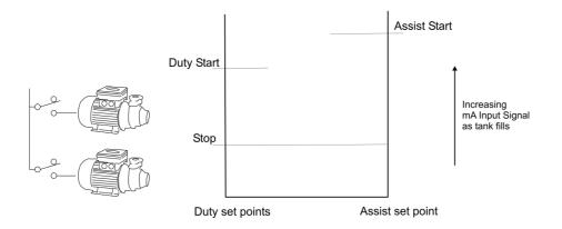
The basic operation outlined in this section can be extended by selecting additional parameters in the software menu (see section 5), this greatly increases the 920 functionality.
