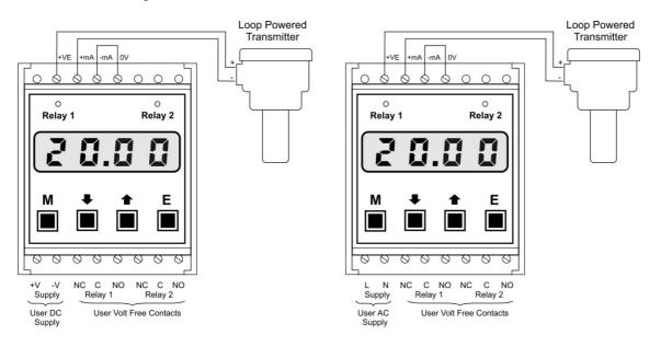
Although not essential it is recommended to connect the initial duty pump to relay 1 contacts and the assist to relay 2, this makes the logic easier to understand during commissioning etc. For more demanding applications that require additional relay outputs multiple 920s or a combination of 920 and 900 trip amplifiers can be used by connecting the transmitter loop in series as follows.
