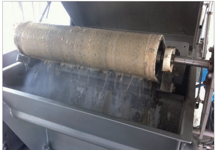
Hydro MicroScreen™ rotating belt reduces BOD and gets more TSS
