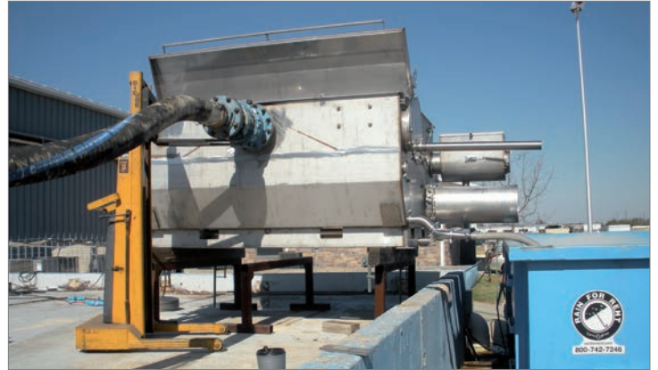
Small footprint Hydro MicroScreen™ system
