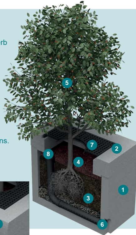
Figure 1 - The Hydro Biofilter™ Bioretention System
