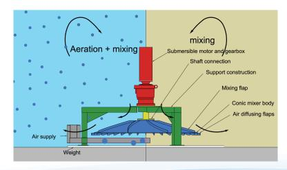
The AER-GS is the ideal combination of an aerator and a mixer. It can be used as an aerator and a mixer together, or it can be used as a mixer only.
