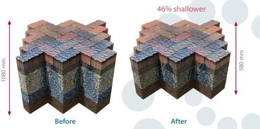
These diagrams are for illustration purposes only; each design is application specific. The above depth example is based on a loading requirement of up to 7.5 tonnes on ground with a CBR of 2%
