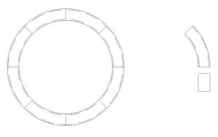
Dimensions Internal diameter 2400mm, External Diameter 3000mm
