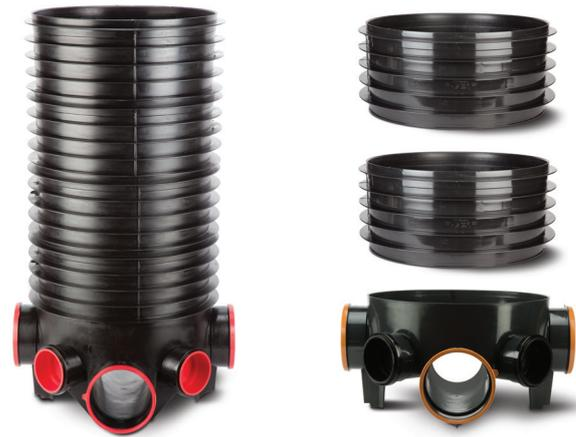
Polysewer Inspection Chambers are sold in component parts to be assembled on site. The base units are connected to Polysewer pipes, then side risers are used to build the chamber to the necessary height and can easily be cut to the correct level using a fine tooth saw. A seal ring is used to ensure a leak tight joint. Cover and frames are available in a range of load classifications.
