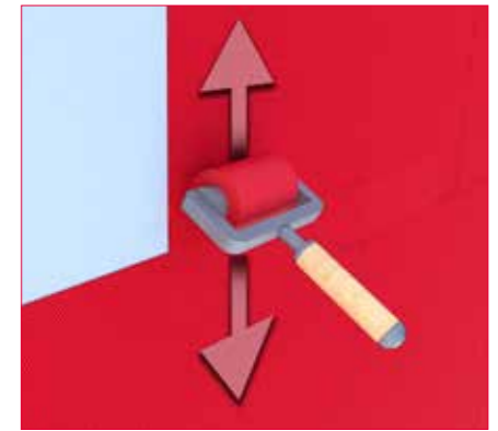
Fig.2 Roll Wraptite to release air bubbles and ensure membrane is well adhered.
