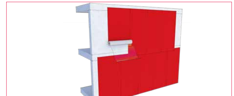
Fig.3 Staggered vertical installation of Wraptite membrane.
