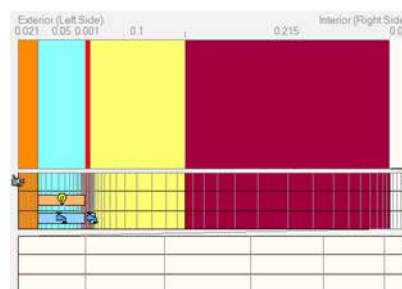
Rainscreen Brick Wall with external PIR/Rockwool
