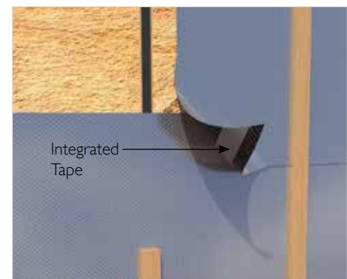
Fig.7: Reflectatherm Premier: Integrated Tape overlap detail
