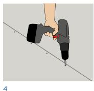
Drill the marked substrate using a 6 mm drill bit and once drilled insert the appropriately sized plug. (6 mm = red plug).
