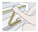
Trim tread material lengths to respective Stair Nosing width. Working a step at a time from the top of the stair downwards, peel off release paper from adhesive in channel(s).
