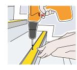
Starting with the first Nosing on the top step, press down and screw into position, then continue down the stairs (1" number 6 screws are recommended). Then fill in the drill holes with plugs.
