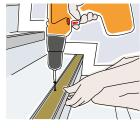
Starting with the first Nosing on the top step, press down and screw into position, then continue down the stairs. (1" number 6 screws are recommended).
