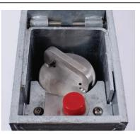
The RetractaPost-GL offers a highly effective and robust way to protect premises and vehicles. The RetractaPost-GL is raised and lowered vertically and is 745mm tall when raised. When lowered the post is fully below ground and covered using the integral lid. The post is lockable in the raised position by rotating the post 45° and then pressing the high-security push button 7-pin security lock. The post is unlocked using the supplied key, rotated and then lowered.
