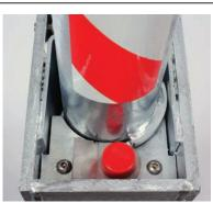
The RetractaPost-GL offers a highly effective and robust way to protect premises and vehicles. The RetractaPost-GL is raised and lowered vertically. When lowered the post is fully below ground and covered using the integral lid. The post is lockable in the raised position by rotating the post 45° and then pressing the high-security push button 7-pin security lock. The post is unlocked using the supplied key, rotated and then lowered.
