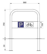
Manufactured from galvanised mild steel; this practical and durable stand is ideal for busy public areas. Supplied galvanised and ragged as standard; flanged, colour coated and stainless steel versions are also available. RAL/BS numbers must be specified at time of order. Reflective tape can be added to maximise visibility.
