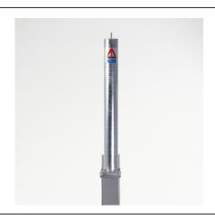
The RGP (removable ground post) offers a highly effective and robust way to protect premises and vehicles. The post is 745mm above ground, when removed the socket is covered using the integral lid. The post is lockable by rotating the post 45° and then pressing the high-security push button 7-pin security lock. The post is unlocked using the supplied key, rotated and then removed.
