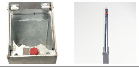
The RGP (removable ground post) offers a highly effective and robust way to protect premises and vehicles. The post is 900mm above ground, when removed the socket is covered using the integral lid. The post is lockable by rotating the post 45° and then pressing the high-security push button 7-pin security lock. The post is unlocked using the supplied key, rotated and then removed.
