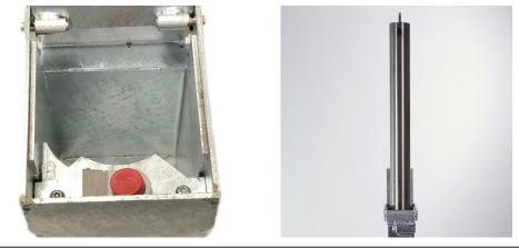
The RGP (removable ground post) offers a highly effective and robust way to protect premises and vehicles. The post is 900mm above ground, when removed the socket is covered using the integral lid. The post is lockable by rotating the post 45° and then pressing the high-security push button 7-pin security lock. The post is unlocked using the supplied key, rotated and then removed.
