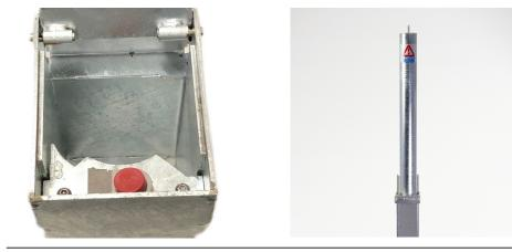
The RGP (removable ground post) offers a highly effective and robust way to protect premises and vehicles. The post is 500mm above ground, when removed the socket is covered using the integral lid. The post is lockable by rotating the post 45° and then pressing the high-security push button 7-pin security lock. The post is unlocked using the supplied key, rotated and then removed.
