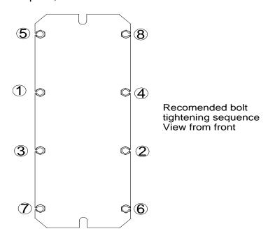
The correct tightening figure is checked by measuring the distance between the moveable front plate and the fixed rear chassis plate and should be calculated as follows:
