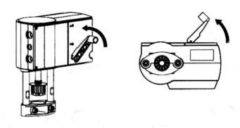
On AVM234 actuators, both LEDs will flash green then red; this indicates manual override is in operation.
