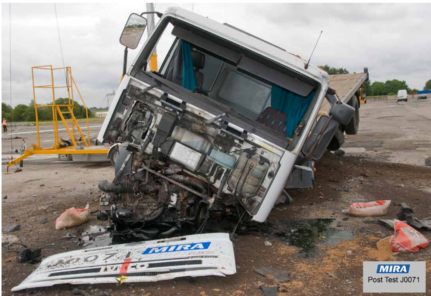
Crash tested in accordance with BSI PAS 68, using a 7.5 tonne N3 lorry traveling at 50mph.
