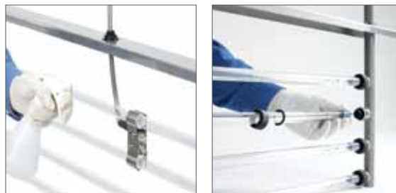
Lightweight, self-contained modules are operator-friendly and make routine maintenance quick and easy. Modules can be individually removed for periodic sleeve cleaning and lamp replacement after 12,000 hours (15 months). An optional, mobile cleaning rack simplifies maintenance procedures.
