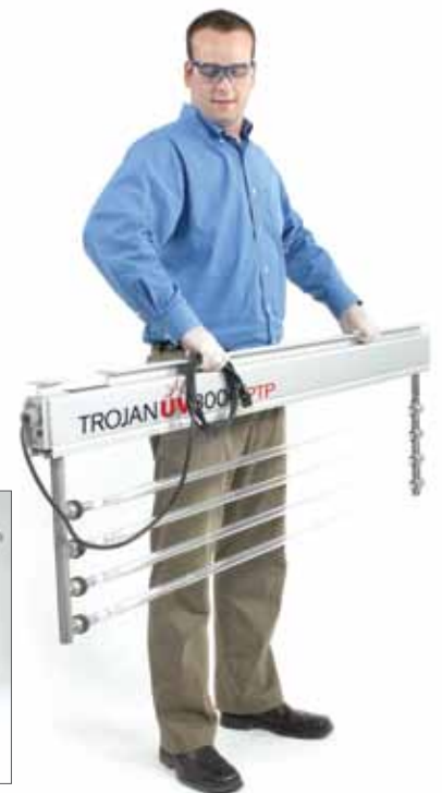
Lightweight, self-contained modules are operator-friendly and make routine maintenance quick and easy. Modules can be individually removed for periodic sleeve cleaning and lamp replacement after 12,000 hours (15 months). An optional, mobile cleaning rack simplifies maintenance procedures.
