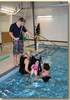
ABOVE: A mechanical hoist offers easy access, suspended from rails over the pool
