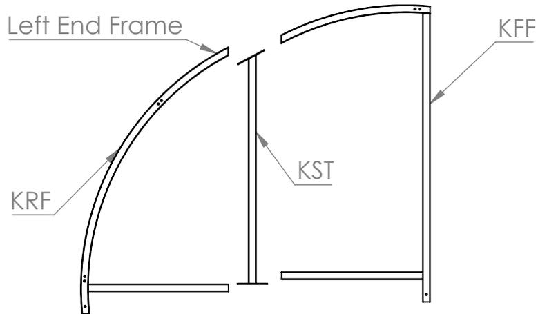
**Note: Shelter ends have 2 sides Left and Right. Make sure all holes are in correct position before assembling.**
