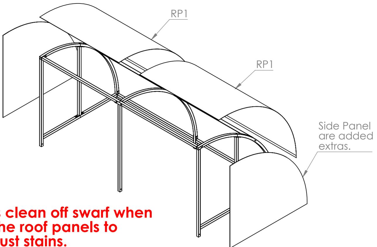
**Always clean off swarf when fitting the roof panels to avoid rust stains.**
