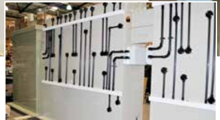
A dosing cabinet ready to be installed in a kiosk. All assembly and testing is conducted at our Service Centre
