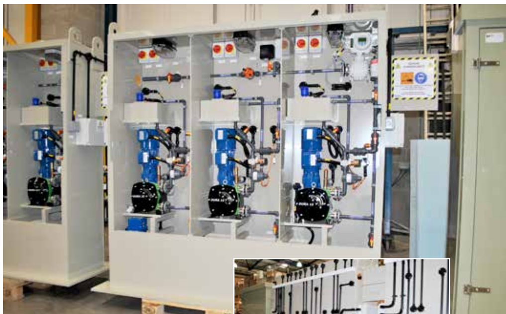
A dosing cabinet ready to be installed in a kiosk. All assembly and testing is conducted at our Service Centre
