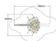
Wet Pour Safety Surfacing 2.6m FFH: 15m<sup>2</sup> x 100mm 2.0m FFH: 22m<sup>2</sup> x 70mm 1.0m FFH: 9m<sup>2</sup> x 40mm
