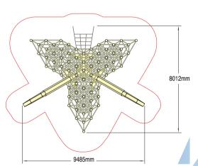
Wet Pour Safety Surfacing 2.0m FFH: 79m<sup>2</sup> x 70mm
